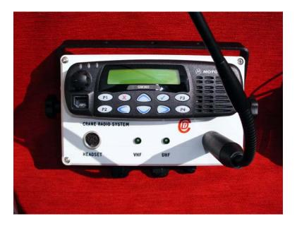
The main equipment is mounted in an IP66 enclosure.
